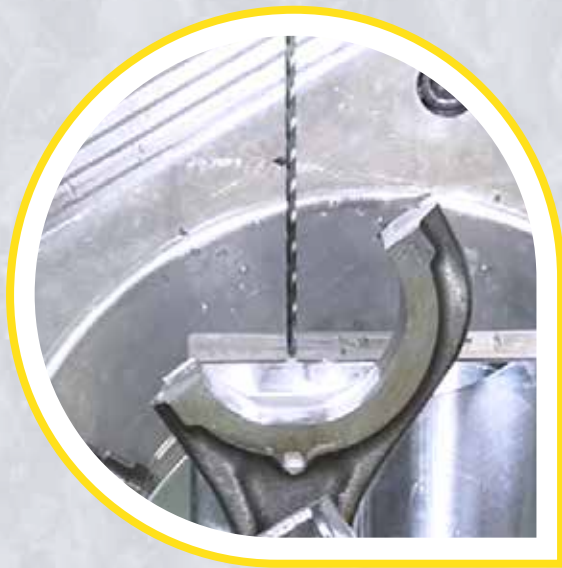
Spiral Channels with Internal Coolant for Efficient Lubrication
